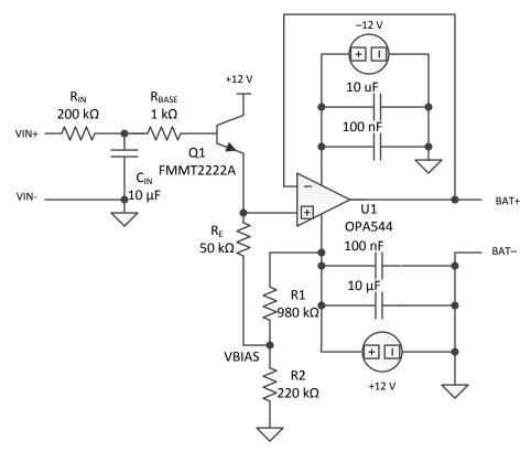
Figure 1. Battery Simulator Circuit
